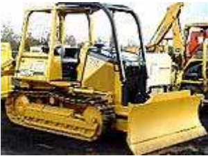
Crawler Tractor with Dozer Blade (model John Deere 450H)
