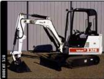
Crawler Tractor with Backhoe (model Bobcat 328)
