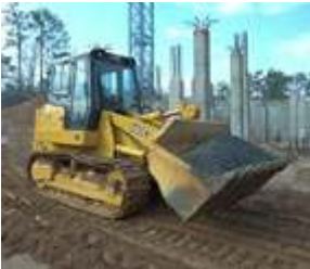
Crawler Loader with Multipurpose Bucket (model John Deere 655 C-T)
